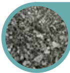
Loose Vermiculite - loose fill insulation
